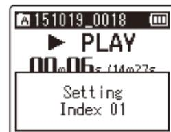
You can set index marks during playback as well as recording, just follow the same process. Up to 200 index marks can be set in a single recording.
